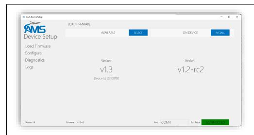
8. Once you have opened the "firmware.afdau" file, the AVAILABLE Version will change from <select file> to the firmware level contained in the selected file and a blue "INSTALL" button will appear on the right hand side of the config tool window.
