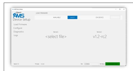
6. Once connected, the port status bar will change to a green CONNECTED message and the ON DEVICE Version will change from <no device> to the firmware level currently on the unit.
