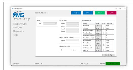
8. To read the configuration from the connected unit, click the green "READ" button. A progress bar will appear, followed by a dialog box telling you the read was successful (or not).
