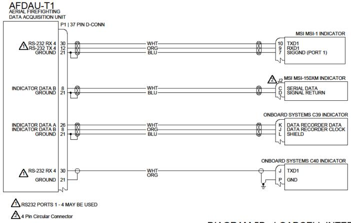
**DIAGRAM 5B - LOADCELL INTERFACES**
