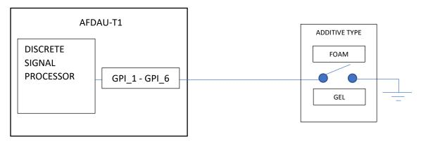
The AFDAU-T1 will always default to WATER or RETARDANT (as selected by the Premix Select discrete, see section 0) regardless of Additive Selection unless an Additive Pump On signal is detected, see section 2.2.6.
