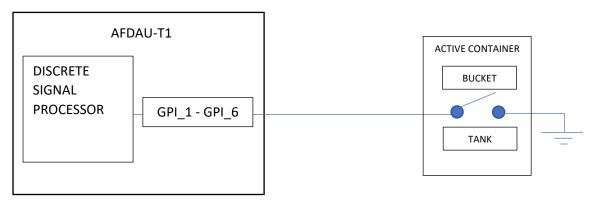
The default configuration when the input is not active is BUCKET type container.
