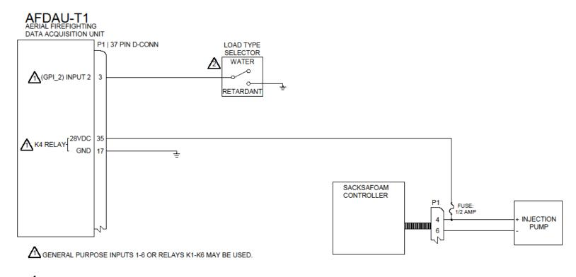
SWITCH OPTIONAL. INSTALL THIS SELECTOR SWITCH IF REQUIRED TO REPORT WHEN THE CONTAINER IS FILLED WITH A PREMIXED RETARDANT.
