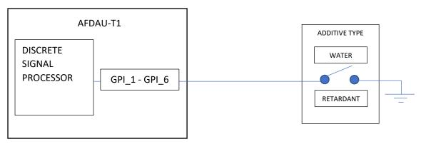
The premix selection will always be overwritten with FOAM or GEL if an Additive Pump On signal is detected, see sections 2.2.5 and 2.2.6.
